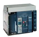
circuit breaker basic frame, Masterpact NT16H1, 42 kA at 440 VAC 50/60 Hz, 1600 A, drawout, without Micrologic, 4 poles
