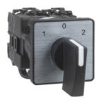
Complete cam switch, Harmony K, changeover switch, 45 x 45mm, 3P, with off position, 45 degree angle, 20A, black marked 2-0-1, screw mounting
